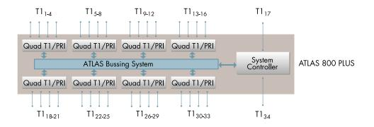
Figure 1-3. Digital Access Cross-Connect System (DACS)
